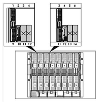
Figure 1 Installing a tape blade adjacent to a half-height Figure 2 server blade.
