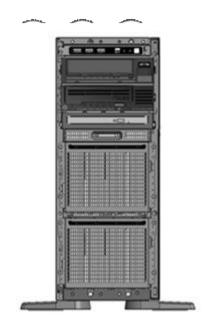
4 LFF hot-plug drive model: Tower - shown without the tower feet.
